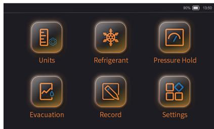
The setting interface includes “Unit Settings,” “Refrigerant Selection,” “Pressure Holding Setting,” “Leak Setting,” “System Setting.” Click the icon to enter the corresponding setting page.
