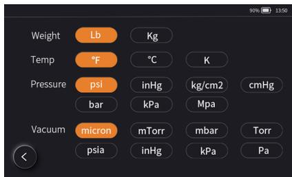
The unit of weight, temperature, pressure and vacuum can be set. Click
