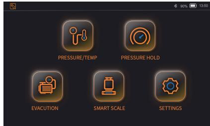
This is the main interface display once the device is turned on. There are “Pressure and Temperature Measurement,” “Pressure Holding Measurement,” “Electronic Refrigerant Scale” and “Setting” for selection. Click on the icon to enter each of the corresponding functions. The status bar on top of the page displayed the time, power/ battery indicator, wireless connection and recording status.
