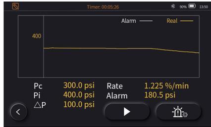
Simply click on the middle of the dial meter to switch to curve mode. Click
