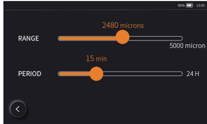
The alarm and duration for refrigerant leak can be set. Click
