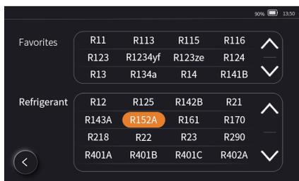
User may select the desired refrigerant from the refrigerant selection box. The selected refrigerant will be added to Favourites automatically. Maximum 20 refrigerant can be added.
