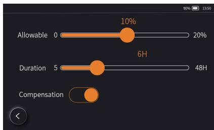
Pressure decay ratio, pressure holding time and temperature compensation can be set in this page. Click
